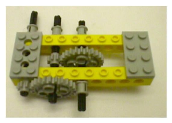
So now the torque at the "output shaft" is 9 times the torque provided on the left ('input") axle. The output shaft will of course spin 9 times slower than the input shaft, but it will be much harder to stall! Of course, once you have discovered a great idea, you might as well keep using it!. Try building an additional stage of gear reduction:
