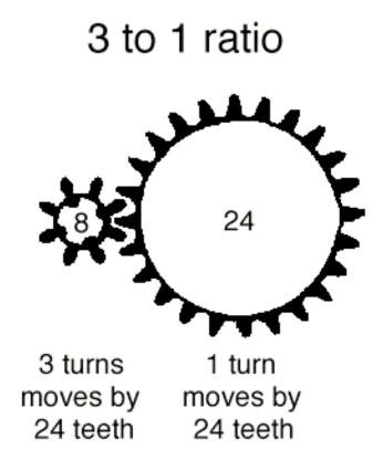
When the 8-tooth gear rotates 3 times, it advances the meshed gear by a total of 24 teeth. Since the meshed gear has a total, it rotates exactly once. (We say this configuration has a 3:1 **gear ratio**.) Thus the 24-tooth gear rotates *three times slower* than the 8-tooth gear.
