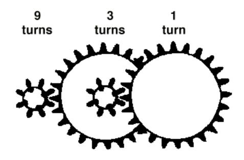
By "ganging together" – or multiplying – two 3to-1 gear reductions, a 9-to-1 output reduction can be achieved. The key is to use intermediary shafts that hold both a large input gear (e.g. a 24-tooth) and a small output gear (e.g. an 8tooth).
