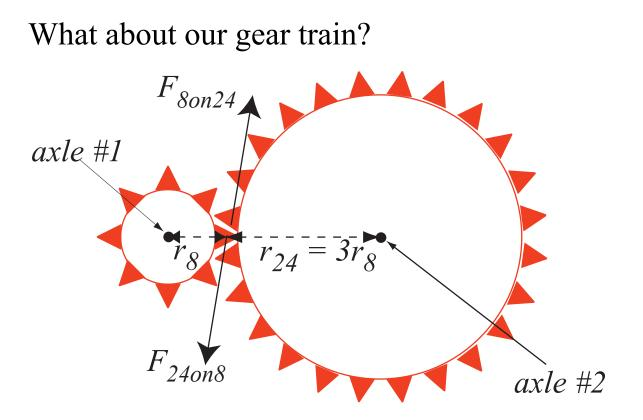
Since torque = r x F, the torque about axle #2 is three times greater than the torque about axle #1; the gear train acts as a **"torque amplifier"**.
