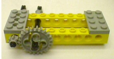
Try rotating the shaft with the small gear with your fingers. Note that the relative rate of rotation of the two axles is different, by a factor of three, which is equal to the ratio of number of teeth on the gears (24:8).
